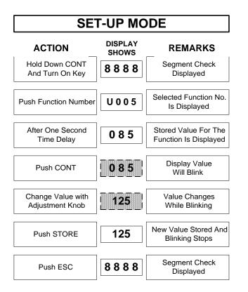
At this point, another function can be monitored/changed by pushing another function number, or the vehicle can be placed in the run mode by holding the **ESC** key down for one second or longer. The display will return to either the diagnostics mode, the BDI display, or a blank display (if BDI is not used and there are no fault codes). The vehicle can now be operated with the Handset connected or the Handset can be disconnected before operation.
