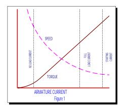
As shown in the typical performance curves of Figure 1, the high torque at low speed characteristic of the series motor is evident.
