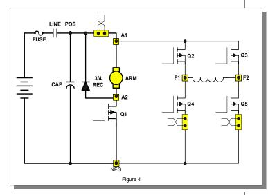
By energizing the transistors in pairs, current can be made to flow in either direction in the field. The field and armature control circuits typically operate at 12KHZ to 15KHZ, a frequency range normally above human hearing. This high frequency, coupled with the elimination of directional contactors, provides for very quiet vehicle operation.
