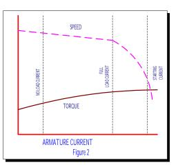
In the separately excited motor, the motor is operated as a fixed field shunt motor in the normal running range. However, when additional torque is required, for example, to climb non-level terrain, such as ramps and the like, the field current is increased to provide the higher level of torque. In most cases, the armature to field ampere turn ratio can be very similar to that of a comparable size series motor (Figure 3.)
